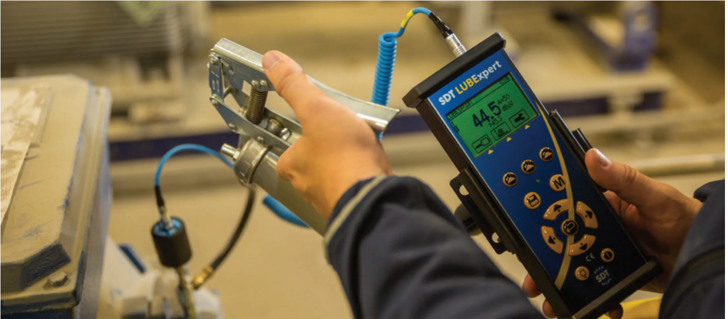
Figure 6: LUBExpert Ultrasound Data Collector & Lubrication Monitoring System
