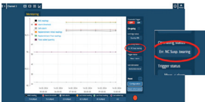
Figure 16: ON-GUARD Dashboard Indicating Suspected Bearing Failure
