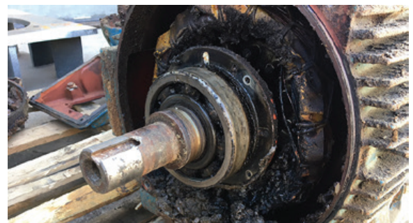
Figure 2: Electric Motor Ruined by Over-Greasing
