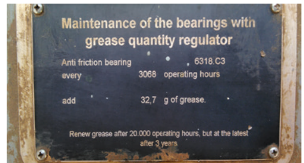
Figure 1: Motor Housing Plate with "Straight-Forward" Re-Grease Instructions
